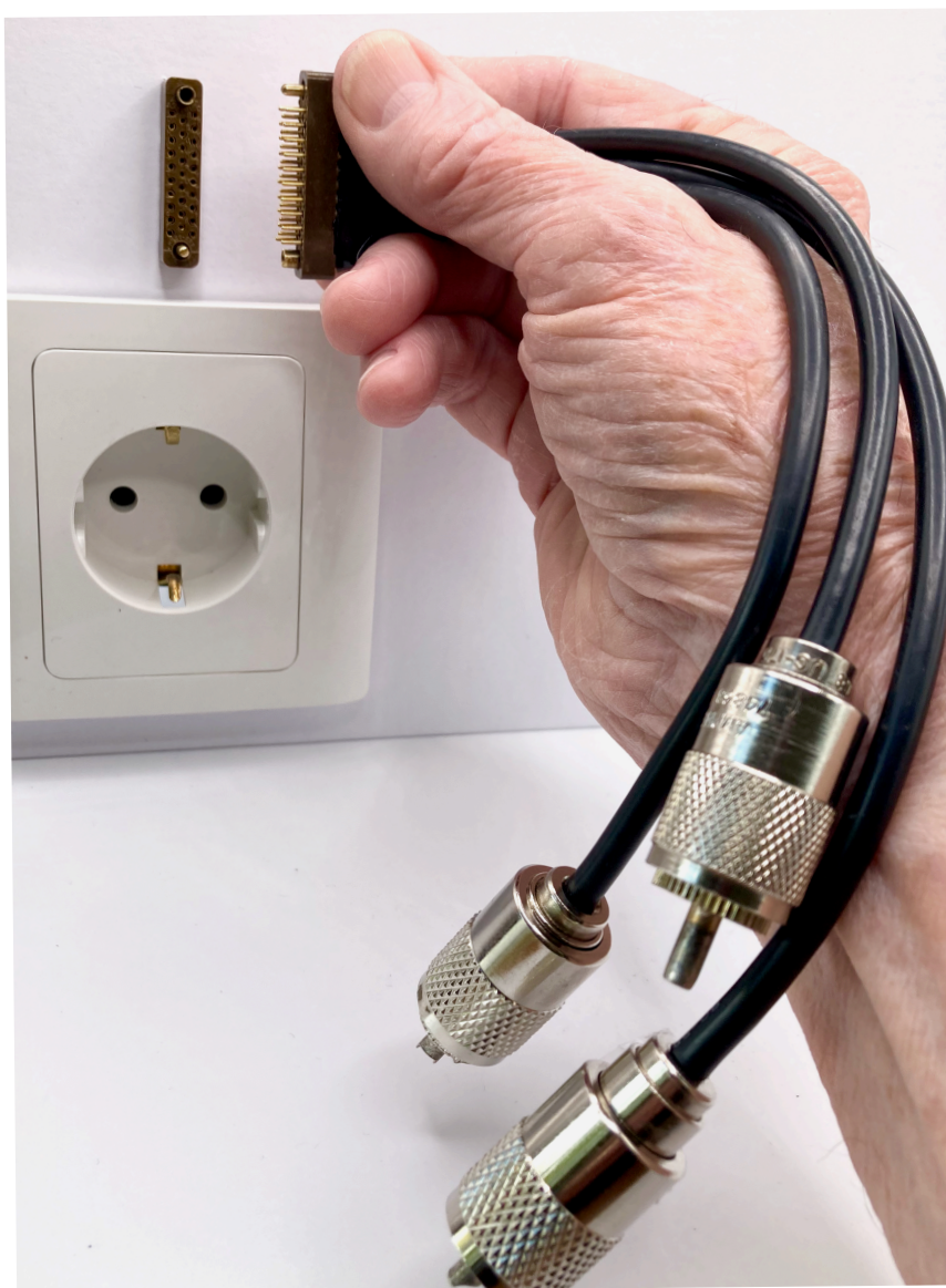
Fig. 3. Replica of patch cable and 29-pin socket on control unit.
